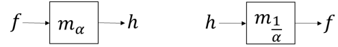
Figure 1-1: The transformation m_\alpha uniquely determines h from f as defined in Eq. (1.2). Similarly, the reconstruction of f from h is m_{1/\alpha} as shown in Eq. (1.3).
