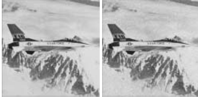
Figure 6. Composite (left) and AWGN channel output (right) images. The composite and channel output images have peak signal-to-distortion ratios of 34.9 dB and 22.6 dB, respectively. \text{DNR} = -12.1 dB, yet all bits were extracted without error. R_m = 1/512 and \text{DNR}_{\text{norm}} = 15.0 dB so the actual bit-error probability is 10^{-6} .
