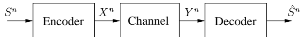
Fig. 1. Authentication system model. The source S^n is encoded to create the channel input X^n , incurring some distortion. The channel models benign degradations due to routine handling, as well as tampering by a malicious attacker. The decoder produces from the channel output Y^n either an authentic reconstruction \hat{S}^n of the source to within some fidelity, or indicates that authentication is not possible.
