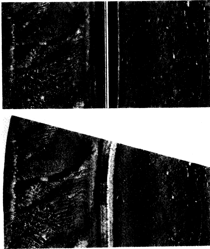
Fig. 21. A second sonograph from our data set, before (top) and after (bottom) correction of geometric distortions. The improvement is most evident in the upper right-hand corner of the image, where features on the bottom appear pronouncedly stretched in the original sonograph, but acquire more natural shapes after processing.
