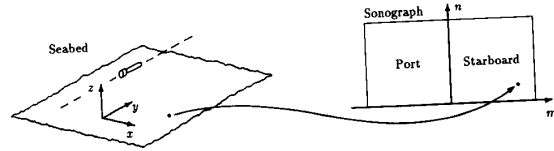
Fig. 5. Coordinate systems defined on the seabed and on the sonograph. The coordinate system defined on the seabed plane may, in principle, have any arbitrary orientation. However, it is useful to align the y direction with the trajectory of the towfish, as shown here, so that it may be referred to as the along-track direction and x as the cross-track direction. In the sonograph, the n direction is defined to point up, coinciding with the direction of scanning, while m is defined to be positive on the starboard (right) side and negative on the port (left) side of the image.
